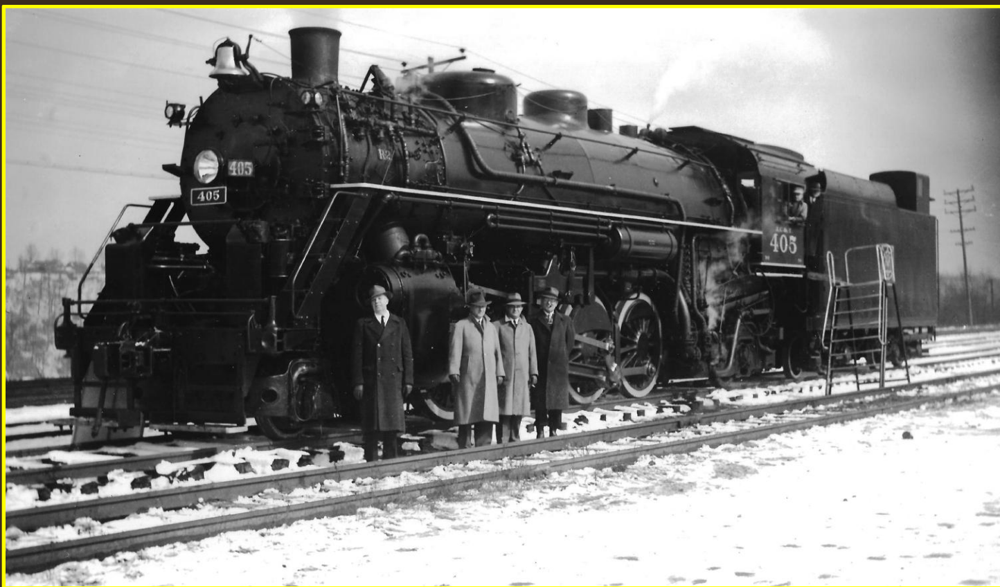
Above: Pride of the AC&Y, two new light 2-8-2's were purchased from nearby Lima Locomotive in 1940 as #404 and #405. Placed in service in February 1941, they were state-of-the-art engines, modern in every way and a symbol of the post-Depression AC&Y. #405 was staged for public viewing at Summit Street in Akron. AC&YHS Archive collection.
